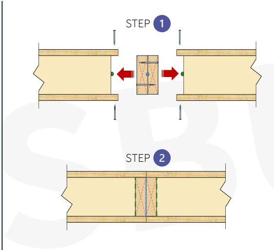
Timber joints to be either: 1 No. Solid Timber or; 2 No. Timbers (nailed and glued). When fully nailing Timbers, Glue is also to be used. NO EXCEPTIONS
