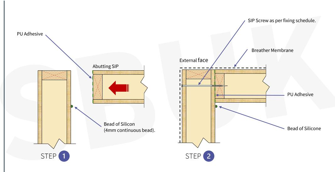
ALL CAPPING TIMBERS FIXED INTO REBATES AS PER DETAIL
